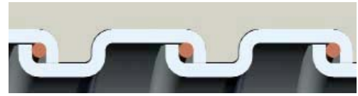
Square-Locked Design with integral bonding wire 3/8" through 1-1/4"
